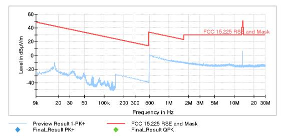
The highest peak is the NFC 13.56 MHz carrier frequency.
