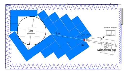
Radiated measurements setup f > 17 GHz:
