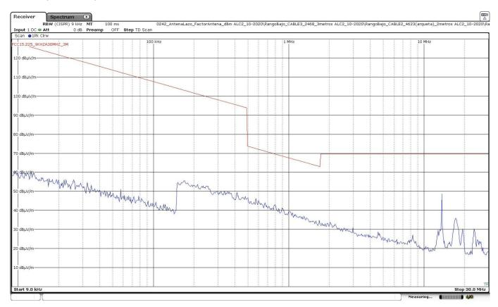
The limits shown in the above plot are extrapolated to 3 meters. The highest peak corresponds to the carrier level.
