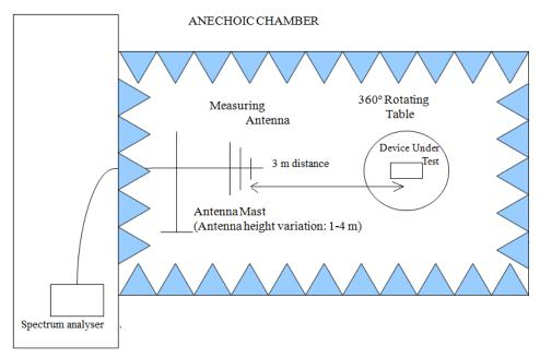
Shielded Control Room For Radiated Measurements
