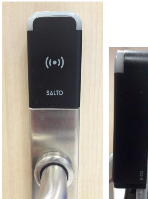
Photo 4: Detail of front view outside part of the door with PPD connection (Portable Programmable Device) and detail of the plastic bottom side edge with Type mark E1722
