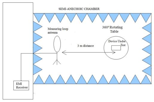
Shielded Control Room For Radiated Measurements
