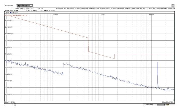
The highest peak is the RFID 13.56 MHz carrier frequency.
