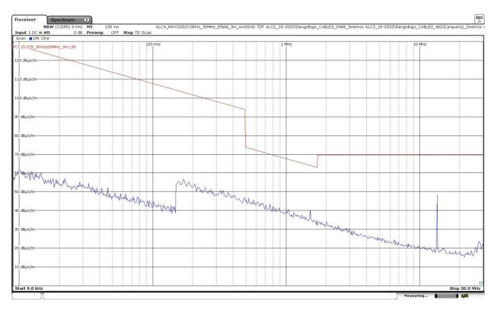
The limits shown in the above plot are extrapolated to 3 meters. The highest peak corresponds to the carrier level.
