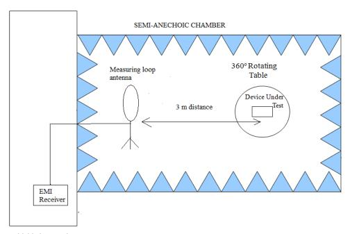
Shielded Control Room For Radiated Measurements
