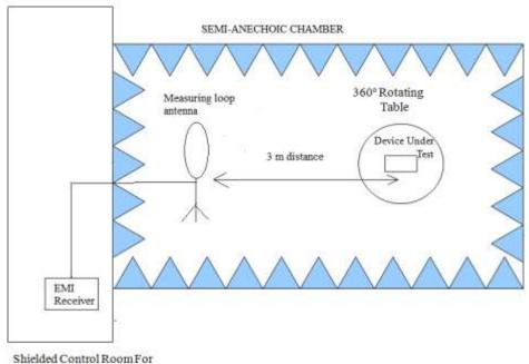
Shielded Control Room For Radiated Measurements
