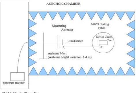
Shielded Control Room For Radiated Measurements
