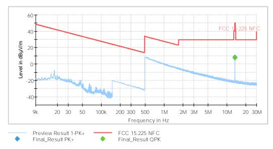
The highest peak is the NFC 13.56 MHz carrier frequency.
