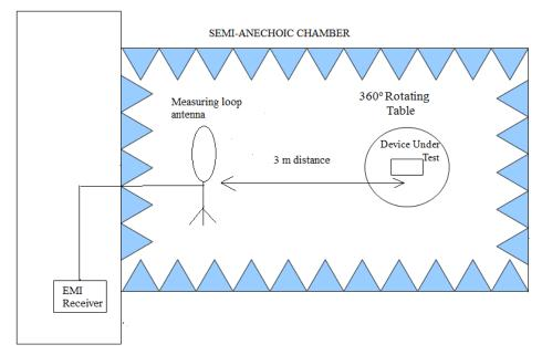
Shielded Control Room For Radiated Measurements
