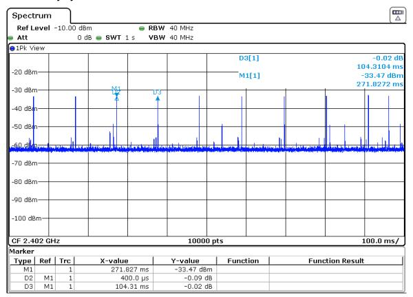
According to ANSI C63.10, paragraph 7.5, we can determinate the Duty Cycle in this way: Duty cycle correction factor  $\delta$  = 20 \* log (Tx ON (ms) \* Number of pulses within 100 ms) / 100 ms  $\delta$  = 20 log (400us)/100ms = -47.97 dB.
