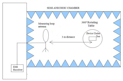
Shielded Control Room For Radiated Measurements
