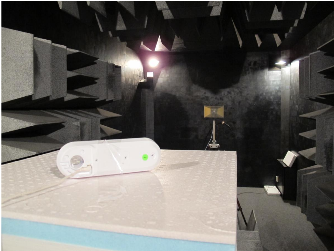
Photograph 1: Radiated emissions test set up, exploratory
