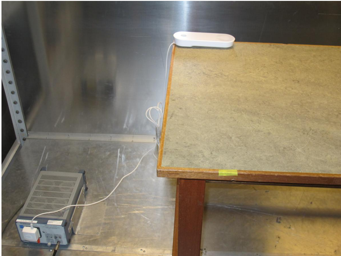
Photograph 4: Conducted emissions test set up
