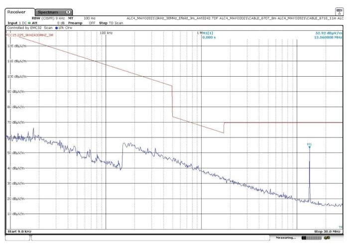
The peak above the limit is the NFC 13.56 MHz ISO 15693 carrier frequency.
