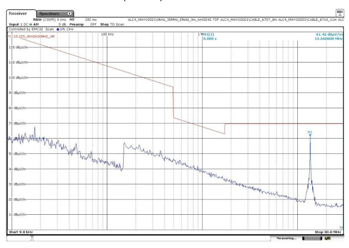
The peak above the limit is the NFC 13.56 MHz ISO 14443A carrier frequency.
