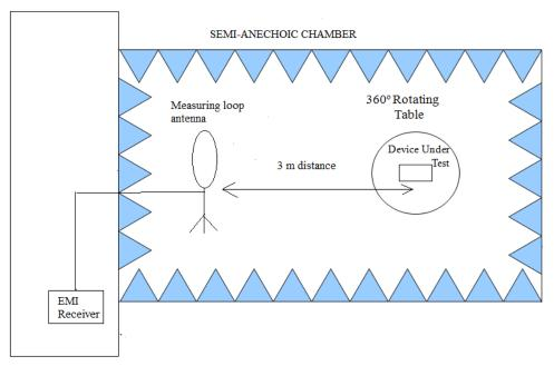
Shielded Control Room For Radiated Measurements
