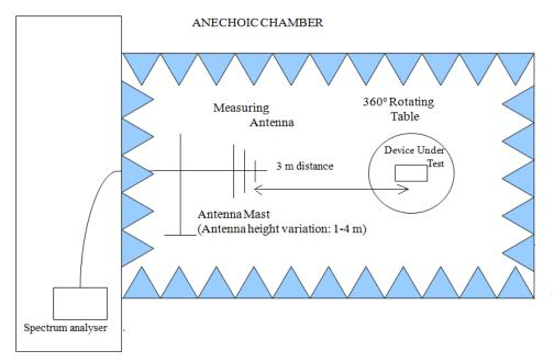
Shielded Control Room For Radiated Measurements
