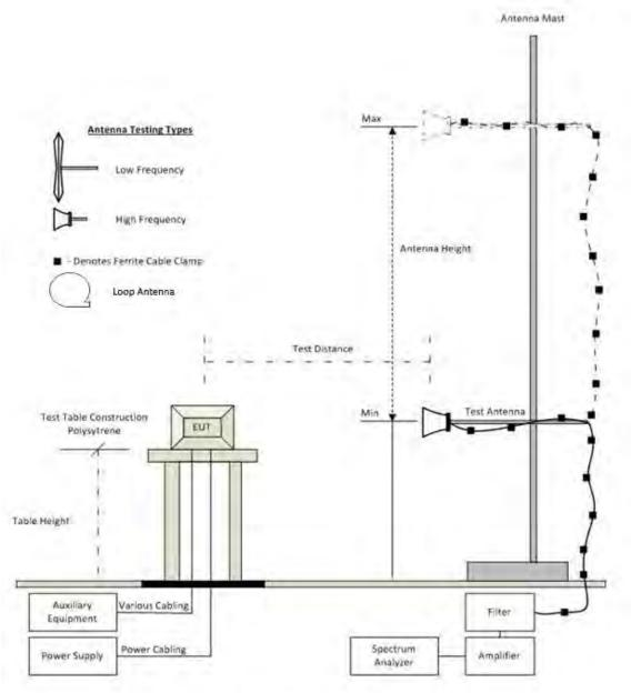
**Radiated Emission Test Setup**
