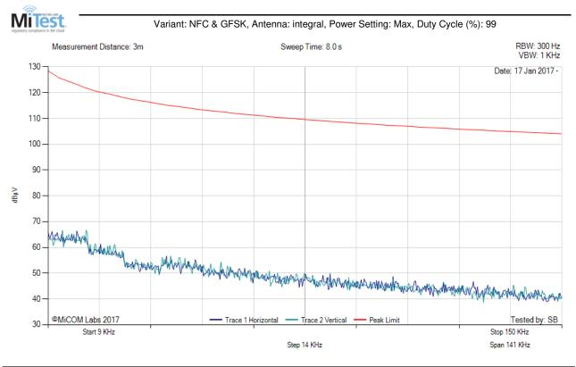
There are no emissions found within 6dB of the limit line. **Test Notes:** NFC & Bluetooth radios are active
