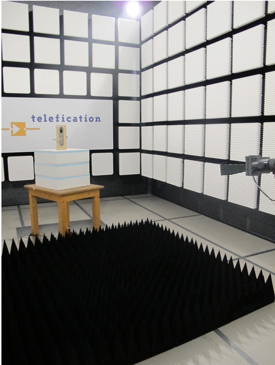
Photograph 3: Test setup radiated emissions 18 - 26 GHz
