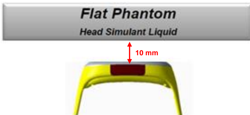
Fig-4.1 Illustration for Smart watch Setup
