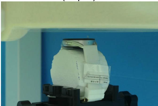
Fig-4.1 Front Face of EUT with 10 mm Gap (Sample C)
