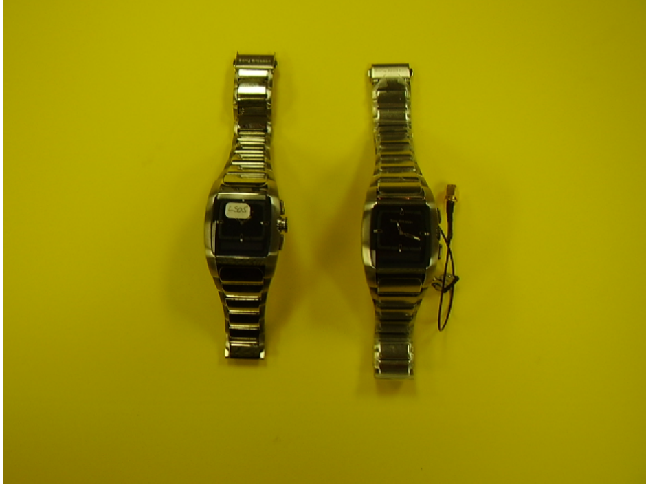
Left: EUT for charging mode Right: EUT for Conducted emissions
