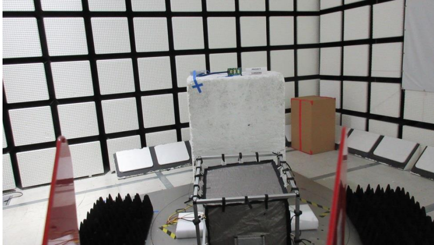
RADIATED FRONT PHOTO (ABOVE 1 GHz)
