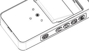
**4.** Put the battery cover back. Make sure the bump on the battery cover is close to the bottom of the radio.
