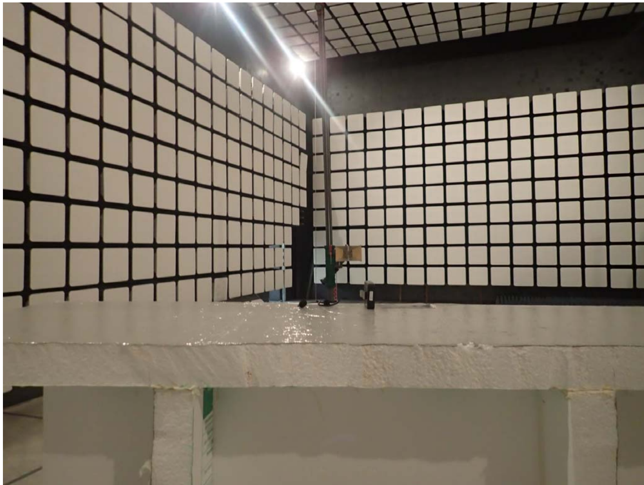
Radiated Emissions @ 3 m, Orthogonal Position 2
