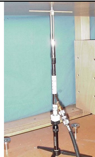
SPEAG 835 MHz Validation Dipole Setup
