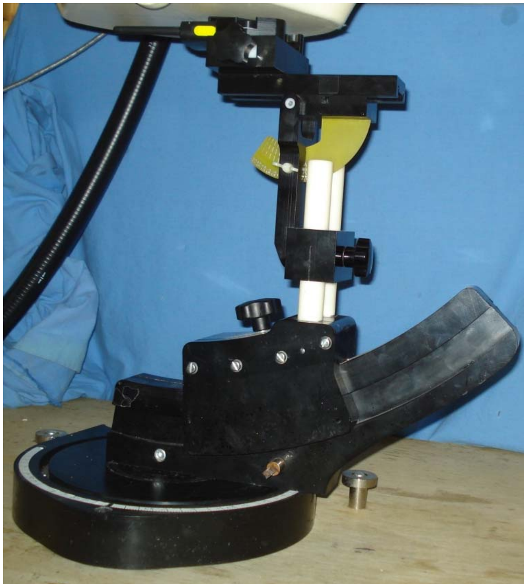
Body-worn SAR Configuration Test Setup with Belt-Clip
