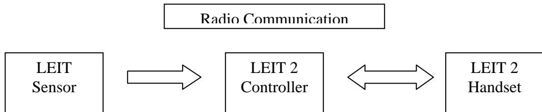
The LEIT ET sensor operates by waking up once every hour and take information measurement to calculate the local microclimate ET. The LEIT Sensor will then send all the different values from each sensor to the LEIT 2 ET controllers or LEIT XRC ETF. The serial ID number will help the LEIT 2ET Controller differentiate between other LEIT ET Sensors in order to take their average to determine more accurate information.
