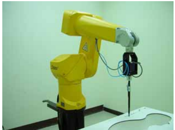
Fig. 5.2 Probe setup on robot
