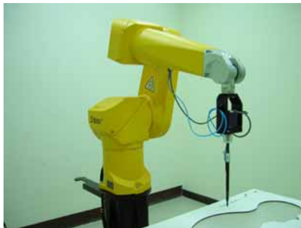
Fig. 5.2 Probe setup on robot
