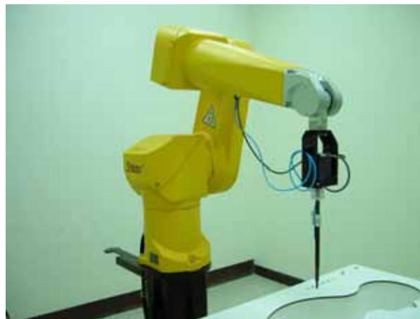
Fig. 5.2 Probe setup on robot
