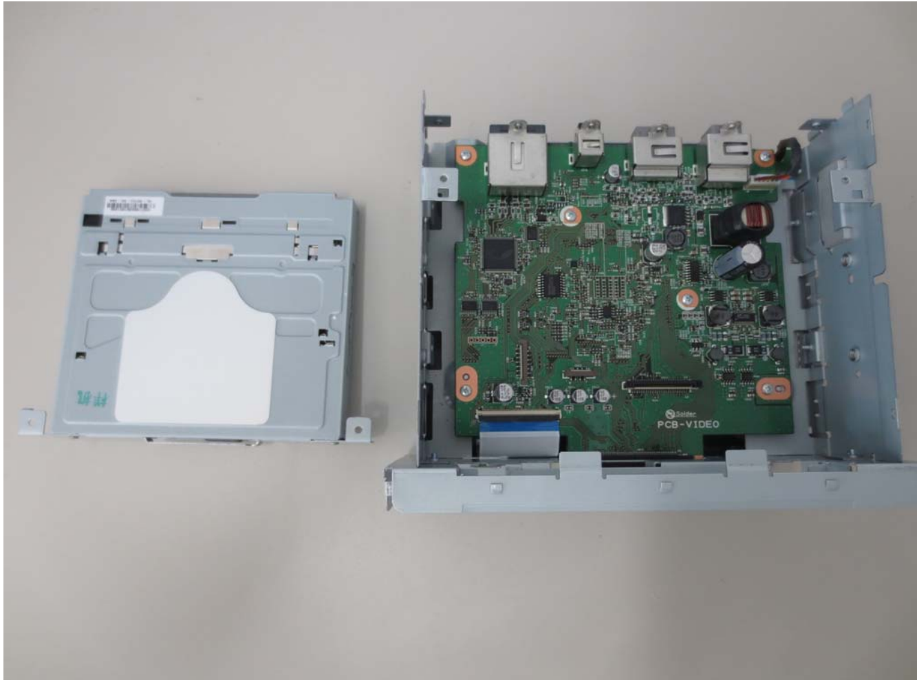
11. Deck is removed.
