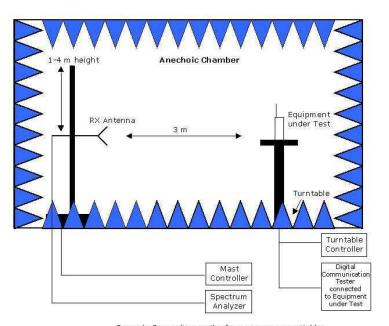
Remark: Depending on the frequency range suitable antenna types, attenuators or preamplifiers are used.
