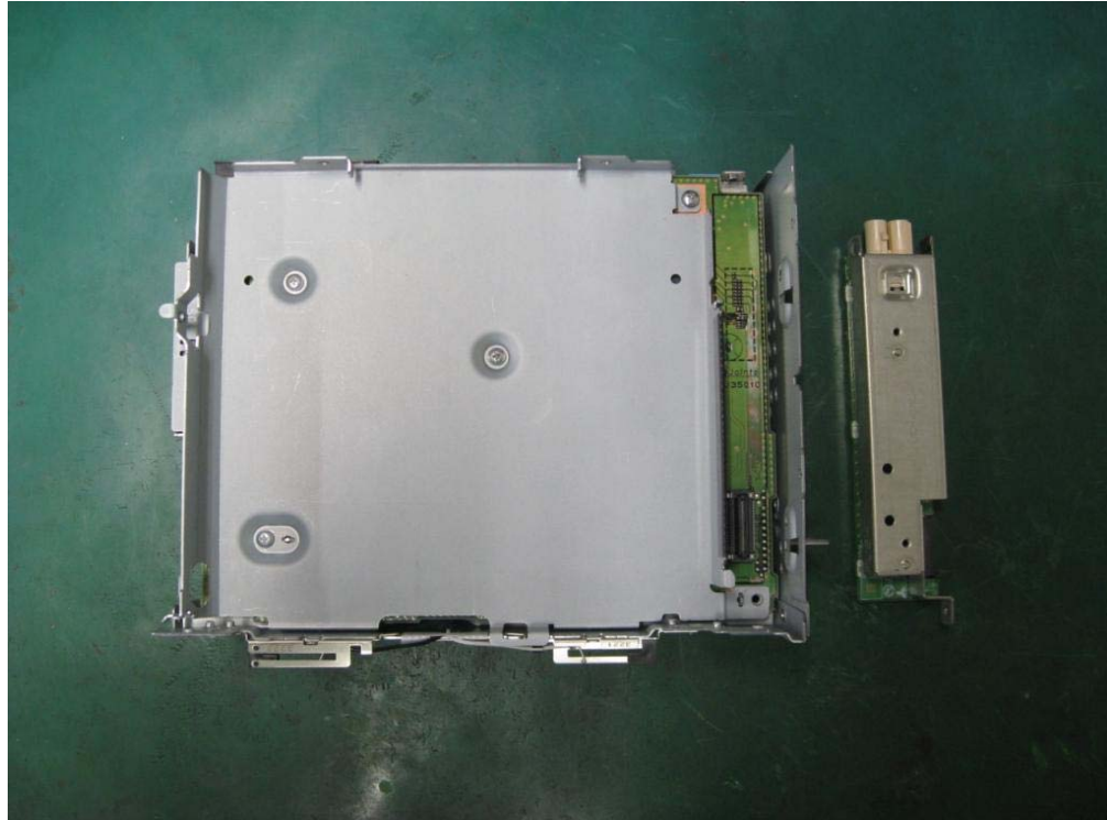
14. PCB-Tuner is removed. Copyright(c) Mitsubishi Electric Corporation
