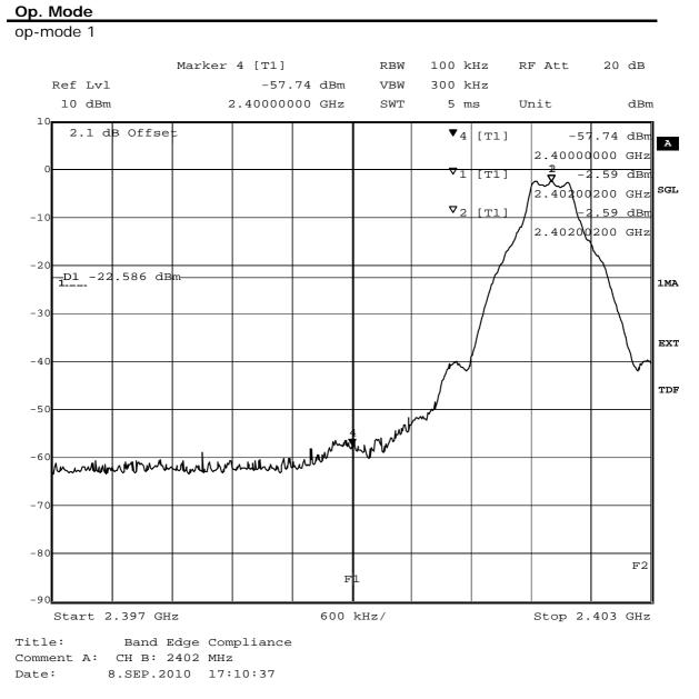
(determination of reference value for spurious emissions measurement)
