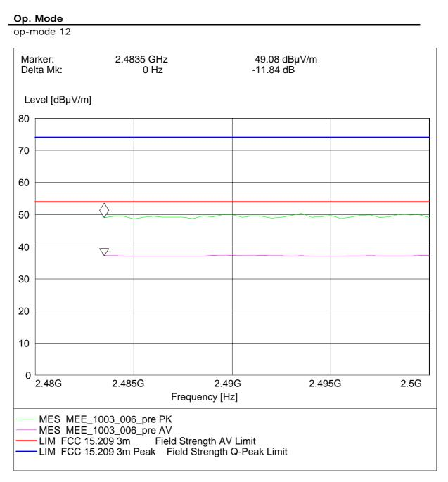
Radiated measurement (higher band edge)
