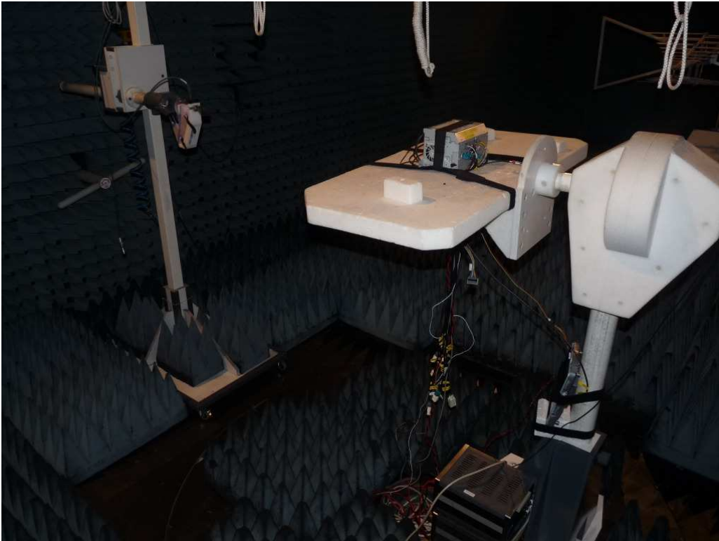
Photo 4: Test setup for radiated measurements (18 GHz up to 25 GHz), FCC15.247
