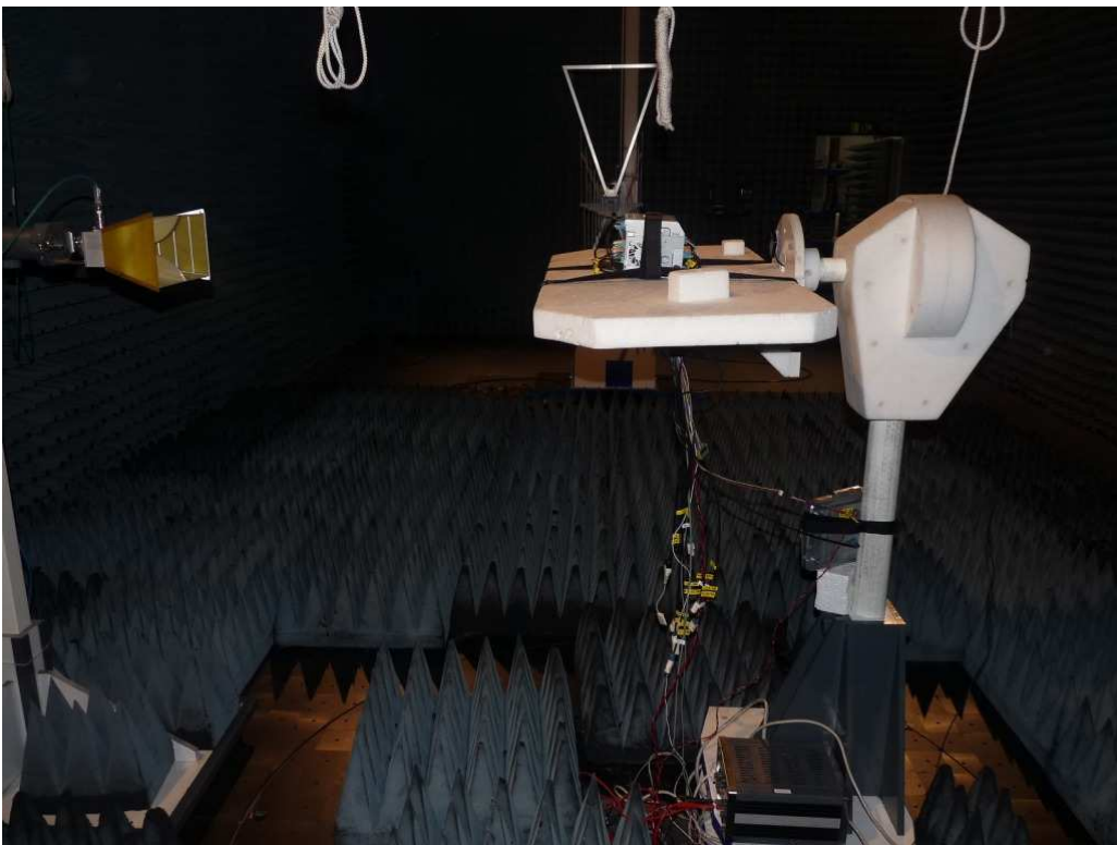
Photo 3: Test setup for radiated measurements (above 1 GHz up to 18 GHz), FCC15.247
