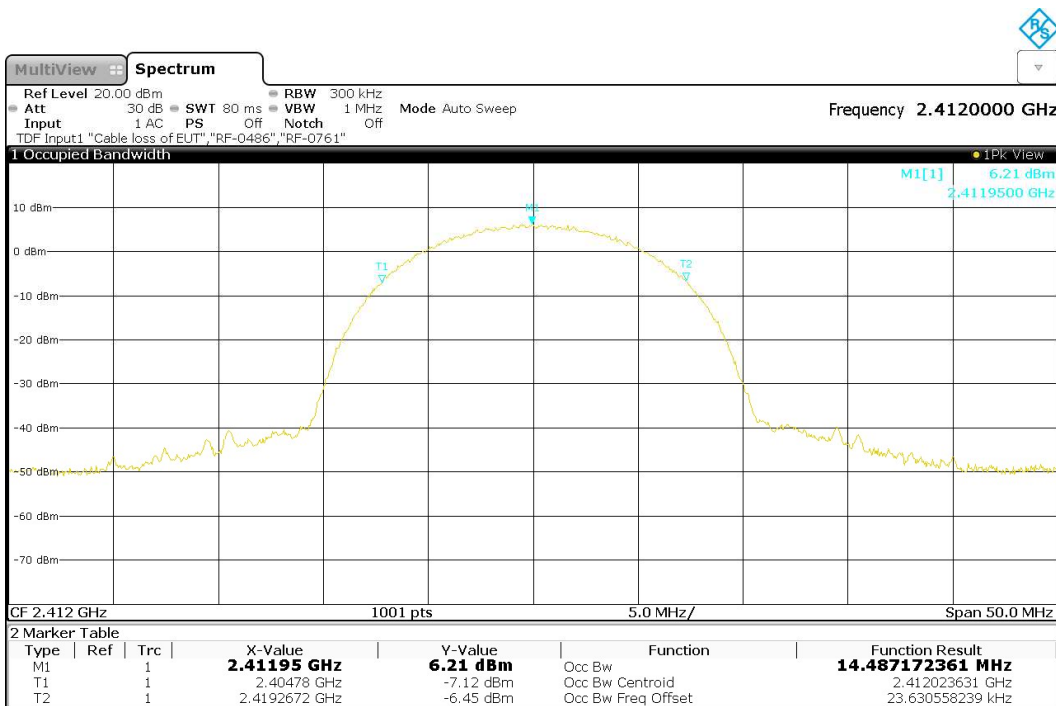
Figure 12: 99% Bandwidth, 802.11b, Mode A (2412MHz)
