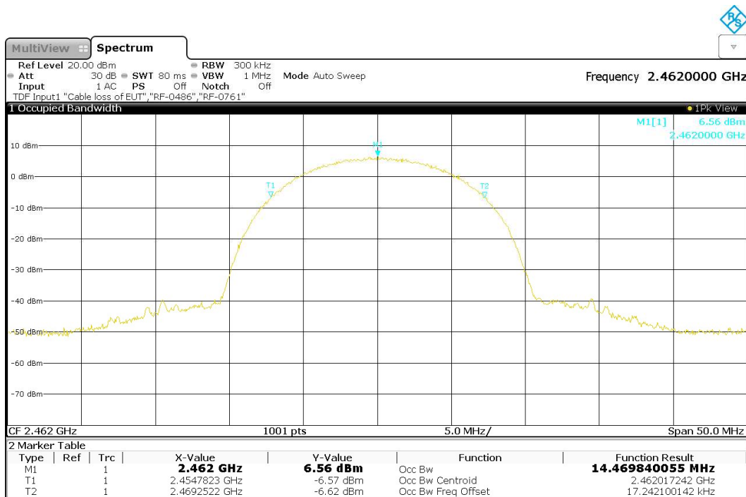
Figure 14: 99% Bandwidth, 802.11b, Mode C (2462MHz)
