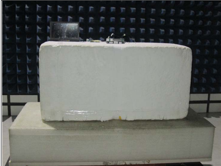
Radiated Emission Test above 1GHz
