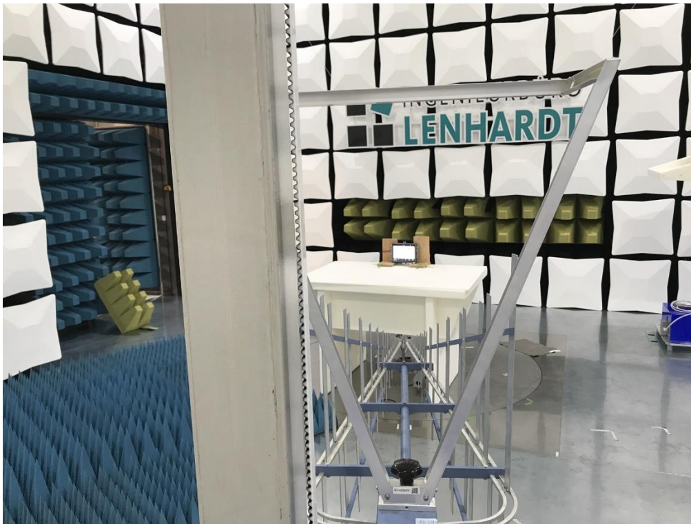
Photograph 1: Radiated emission 30...1000 MHz
