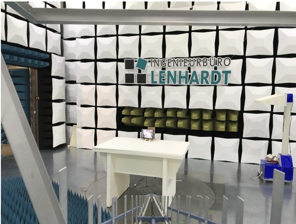
Photograph 7: Radiated emission 30...1000 MHz
