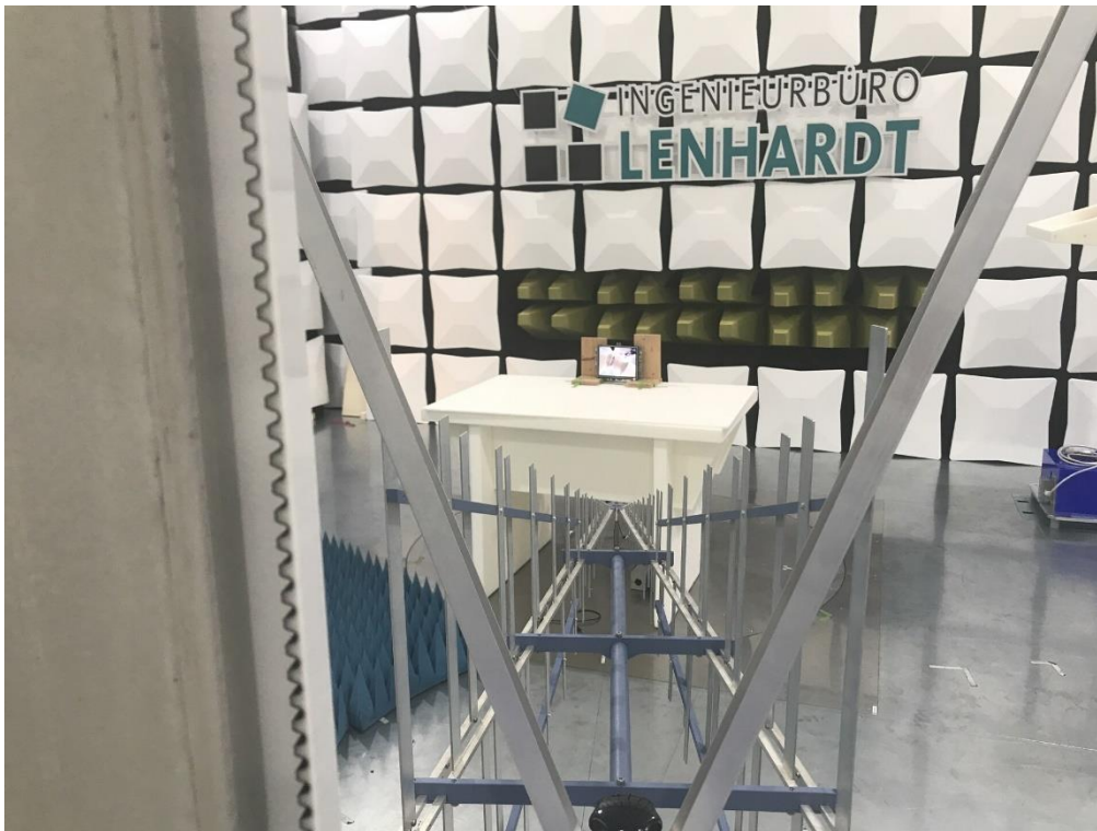
Photograph 4: Radiated emission 30...1000 MHz
