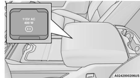
Center Console Power Inverter Outlet
