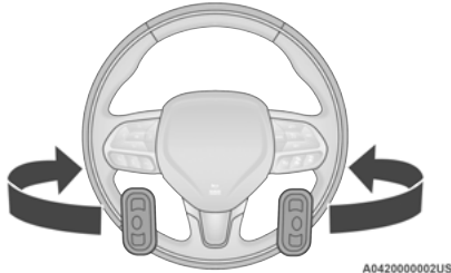
Remote Sound System Controls
