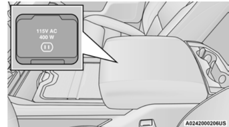
Center Console Power Inverter Outlet
