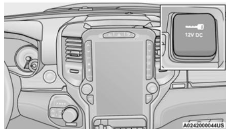
Power Outlet – Top Of Center Stack
