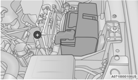
Positive Battery Post
