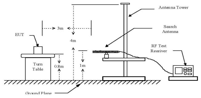
Frequencies measured from 1GHz to 18 GHz configuration
