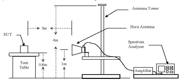
Frequencies measured above 18 GHz configuration
