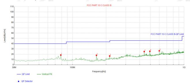
**Suspected List** Freq. Factor Reading Level Limit Margin Height Angle NO. Polarity [MHz] [dB]  $[dB\mu V/m]$  $[dB\mu V/m]$ [dBµV/m] [dB] [cm] [°] 78.548549 -17.2935.86 18.57 21.43 5 40.00 100 Vertical 163.99399 -17.19 35.27 18.08 43.50 25.42 100 186 Vertical -14.42 16.79 Vertical 215.45545 31.21 43.50 26.71 100 145 439.74975 -8.46 33.59 25.13 46.00 20.87 100 151 Vertical -7.29 5 494.12412 33.00 25.71 46.00 20.29 100 192 Vertical 599.95996 -4.9331.45 26.52 46.00 19.48 100 5 Vertical
