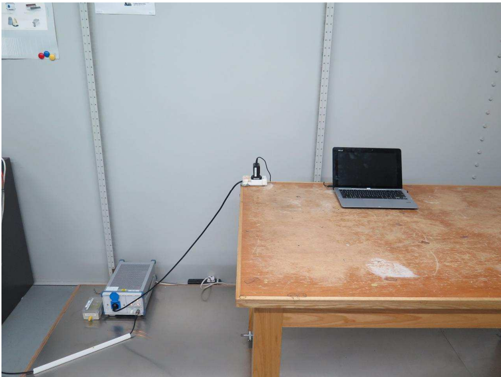
Conducted emission (Front view)
