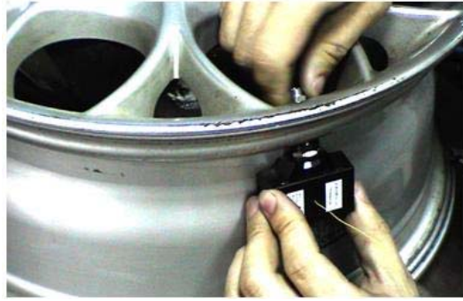
Illustration of sensor installation
