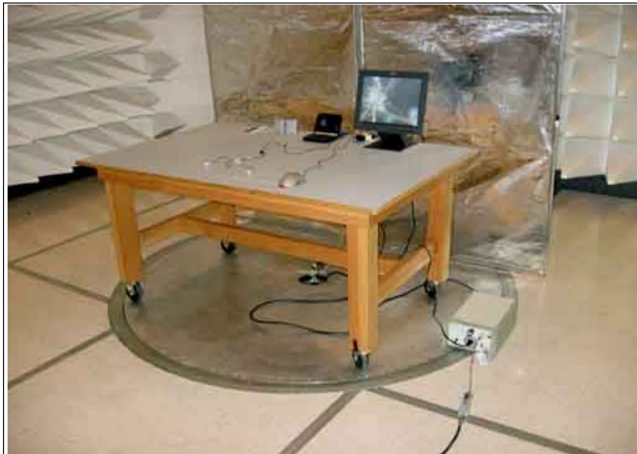
Mains Conducted Emissions - Front View
