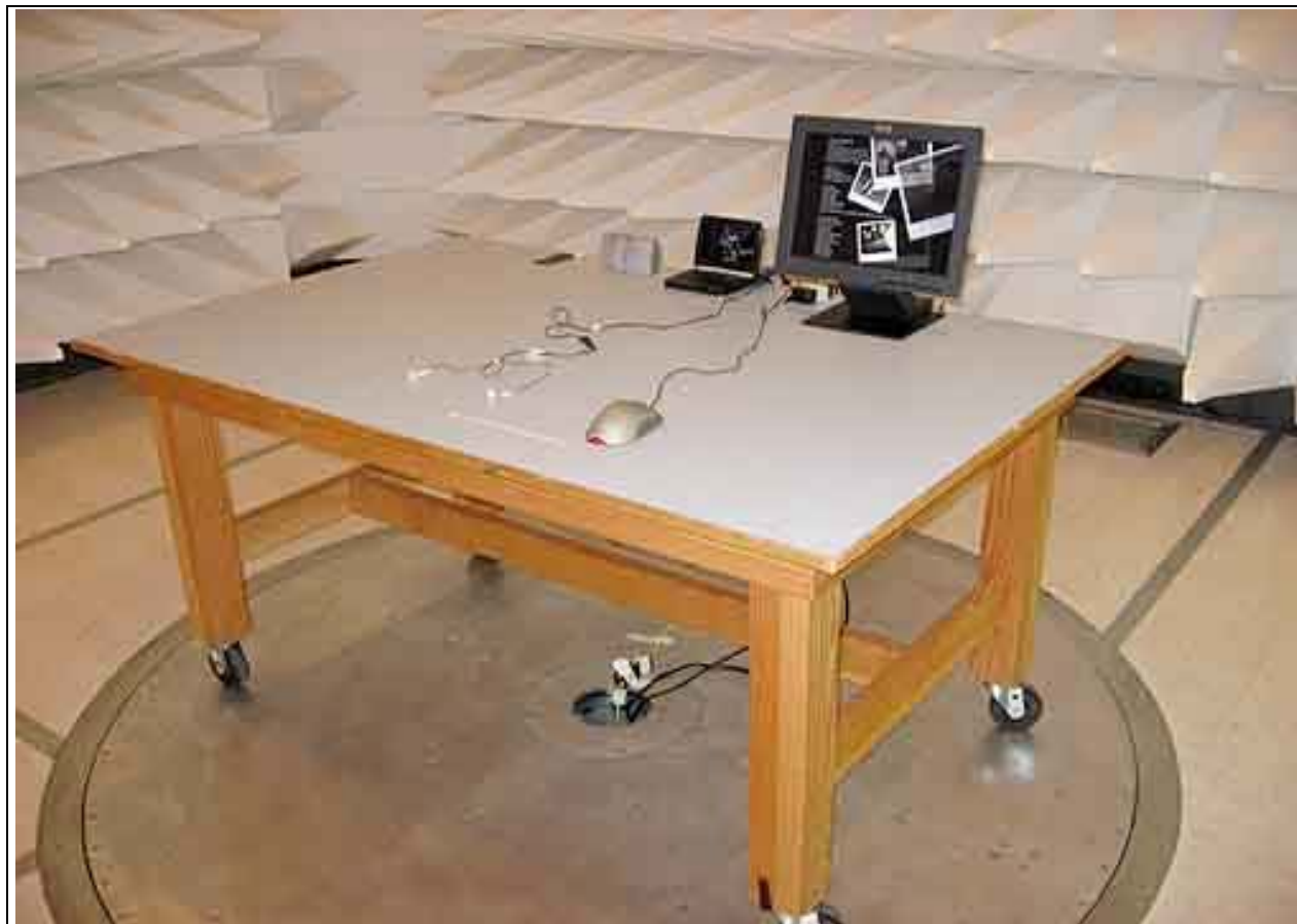
Radiated Emissions - Front View
