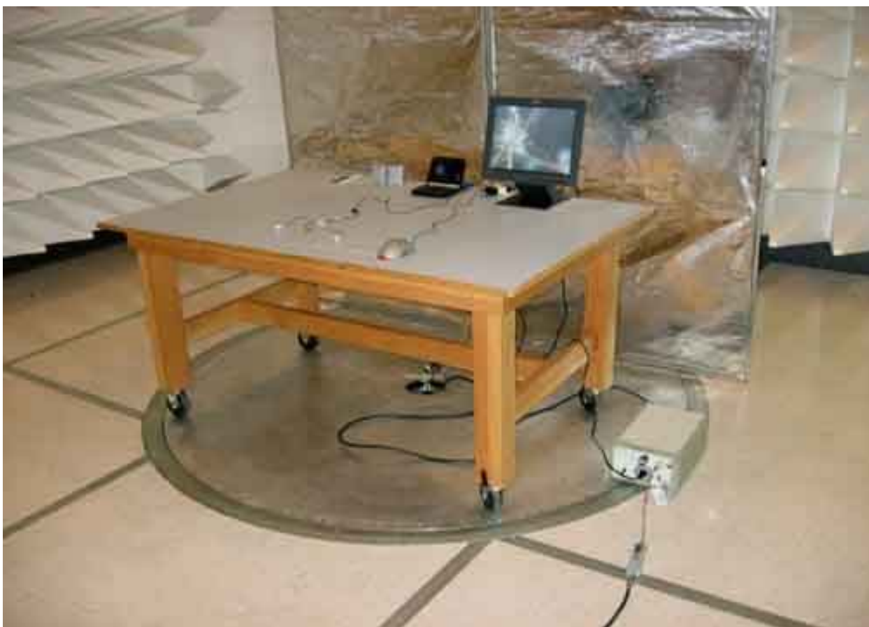
Mains Conducted Emissions - Front View
