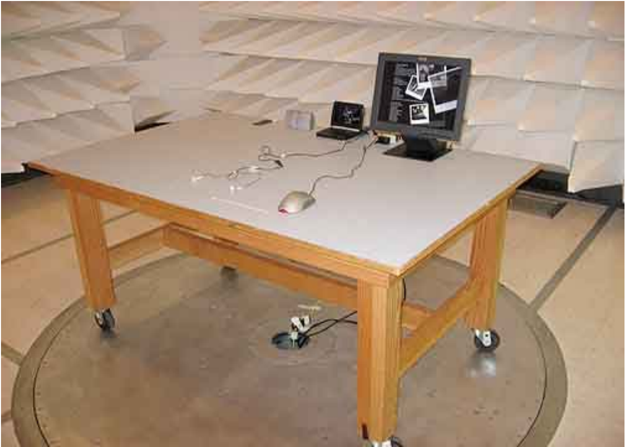
Radiated Emissions - Front View
