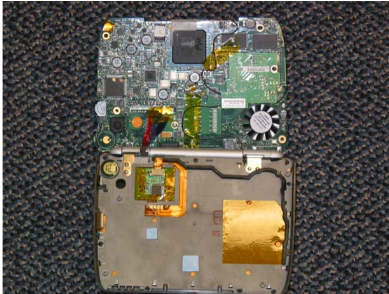
PWB Circuit Side With LAN Module
