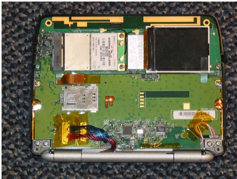
Cover Removed Behind LCD With WAN Module
