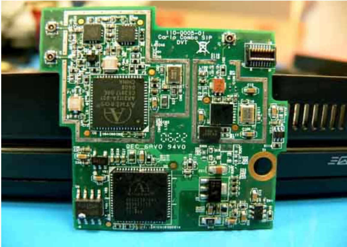
Carlo bottom under RF shields
