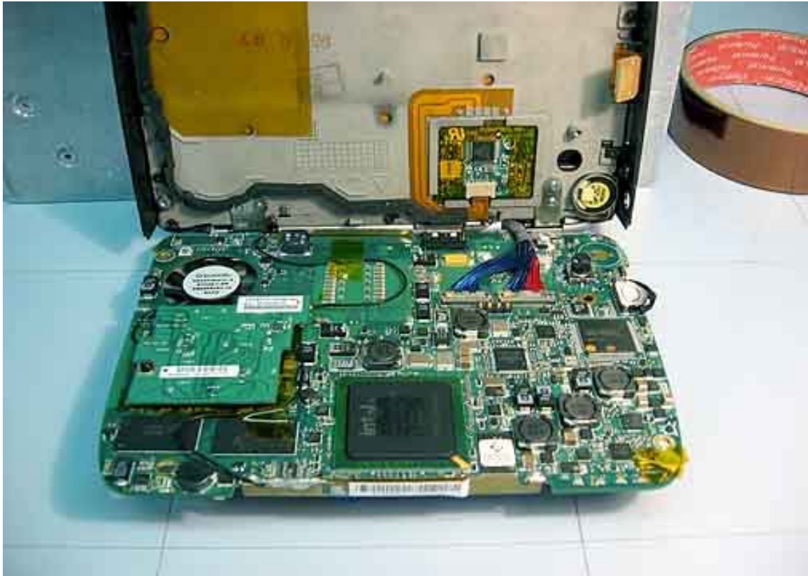
Diversity antenna on front of motherboard
