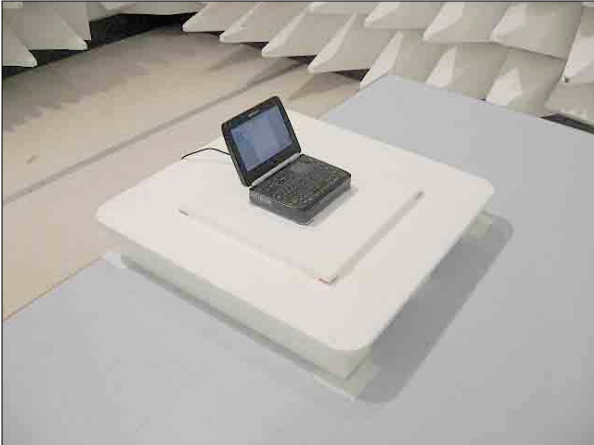
Radiated Emissions – Front View Verification of Radiated Spurious Emissions testing off the Antenna
