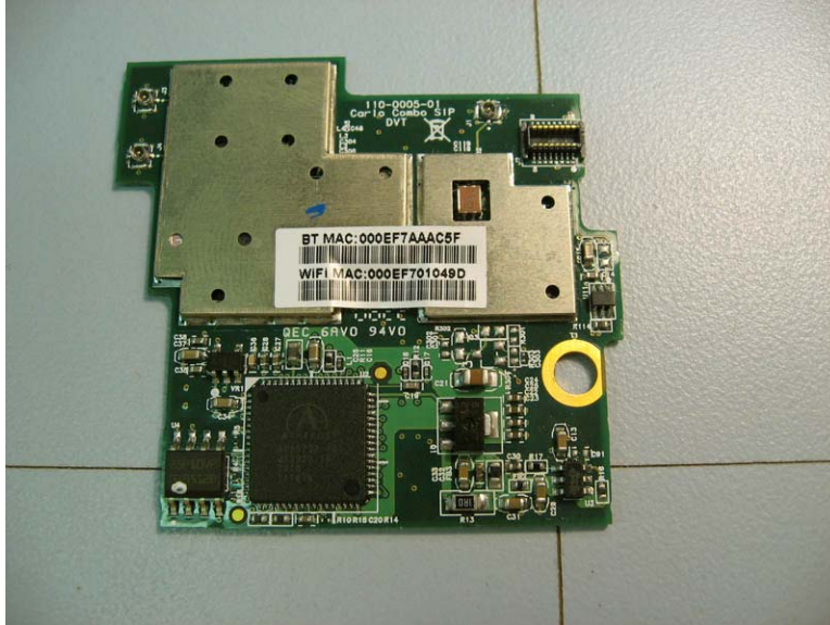
Carlo board bottom - RF shields on
