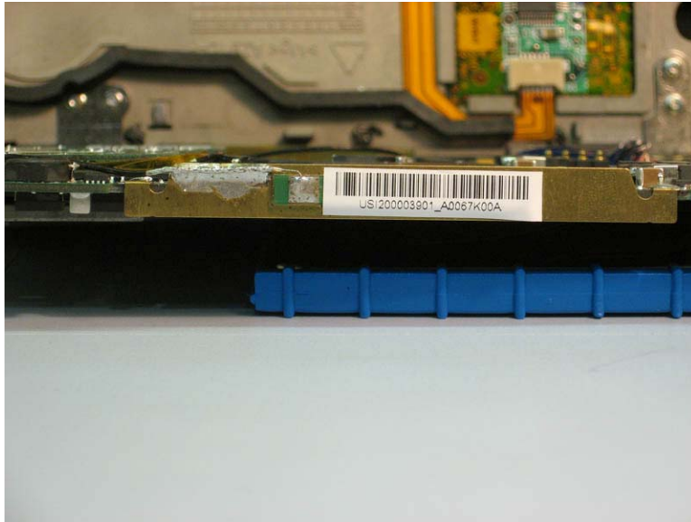
WiFi diversity antenna in front of unit
