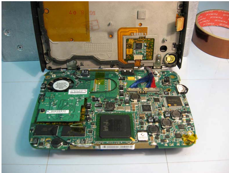
Diversity antenna on front of motherboard
