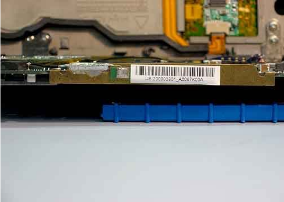
WiFi diversity antenna in front of unit
