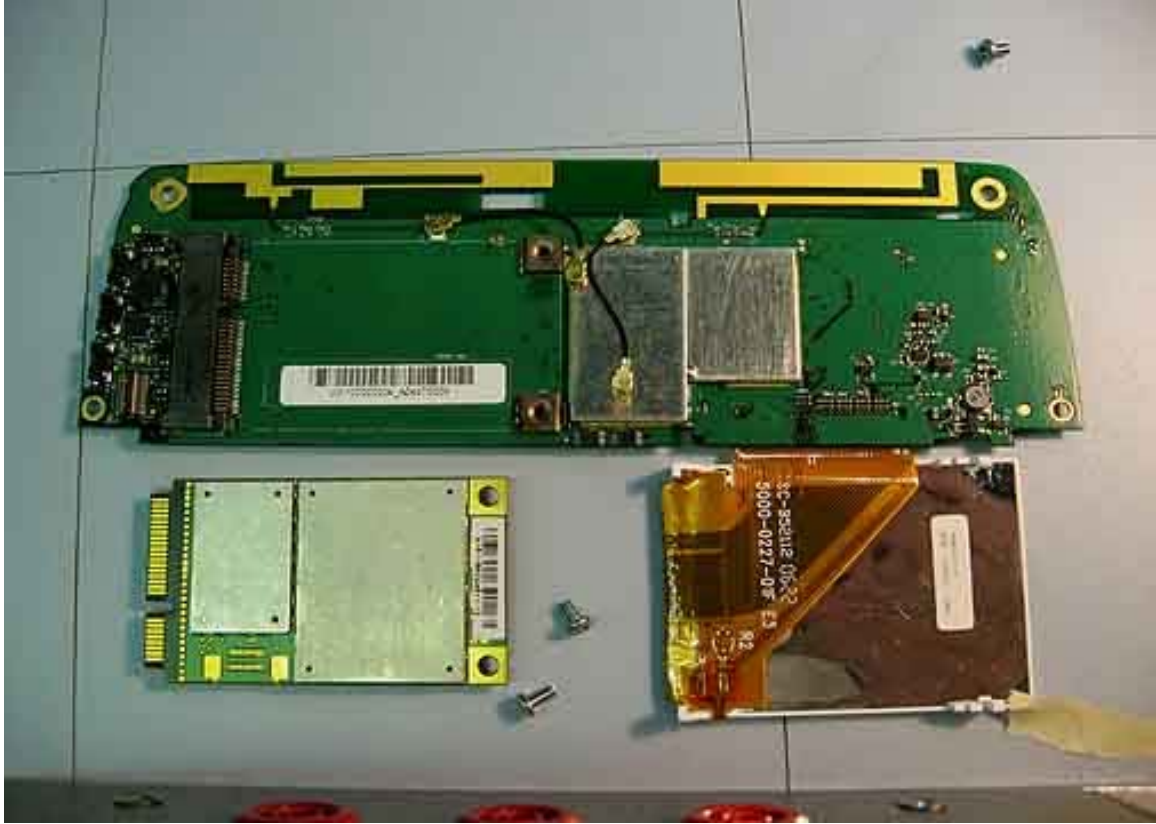
Dino top WAN module and LCD removed
