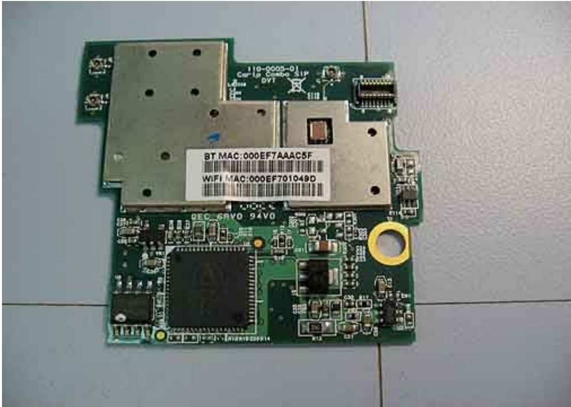
Carlo bottom with RF shields on
